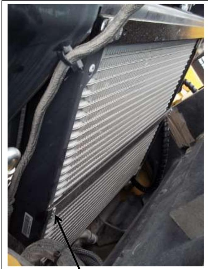
Remove the condenser from the machine and install the rest of the self-drilling screws in the bottom bracket.
