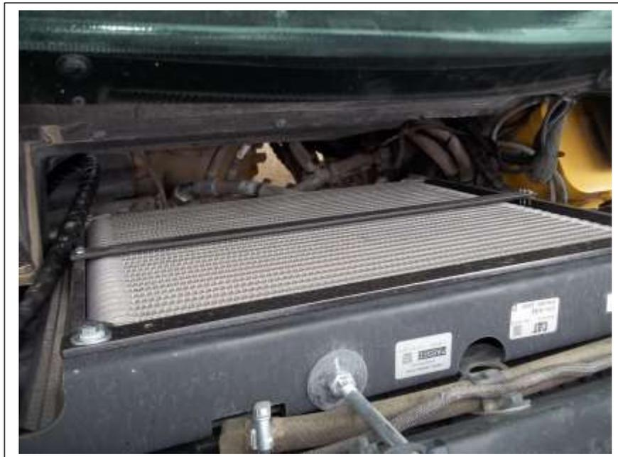
Bolt the top condenser bracket in place across the top of the oil cooler frame. Use the longer M\* bolts provided.
