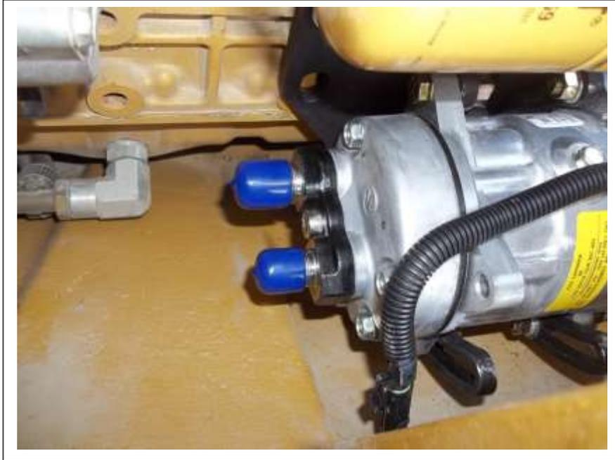
Install the pad fitting onto the back of the compressor. The larger fitting goes on the “S” suction side. The smaller fitting on the “D” discharge side. Ensure both “O” rings are in place and tighten the bolt. This pad can be installed before the compressor is placed in the engine compartment.
