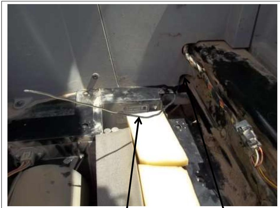
Set the heater box back into place in the cab. Be careful of the drain tubes when setting in place.
