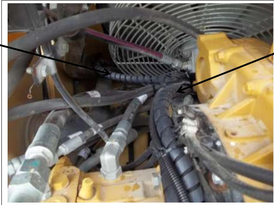
1/2" hose and clutch wire running across the back of the engine and down beside the right side of the radiator fan.
