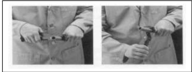
Step 2. Install two proper-sized clips onto the cut end of the hose. Orientation of the clips does not affect the performance of the connection. However, for ease of assembly, both clips should have the same orientation. NOTE: Failure to slide the clips over the hose at this time will require the clips to be stretched over the hose or fitting later. This may permanently damage the clip.
