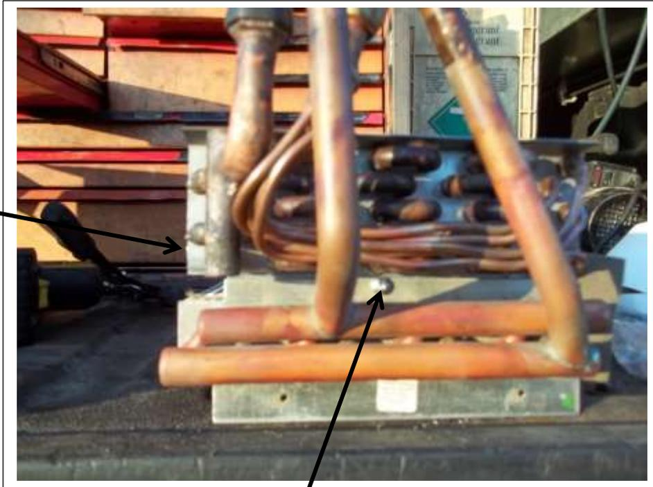
Remove the heater coil from the box and fasten the new evaporator to the heater coil as shown using self drilling screws provided.
