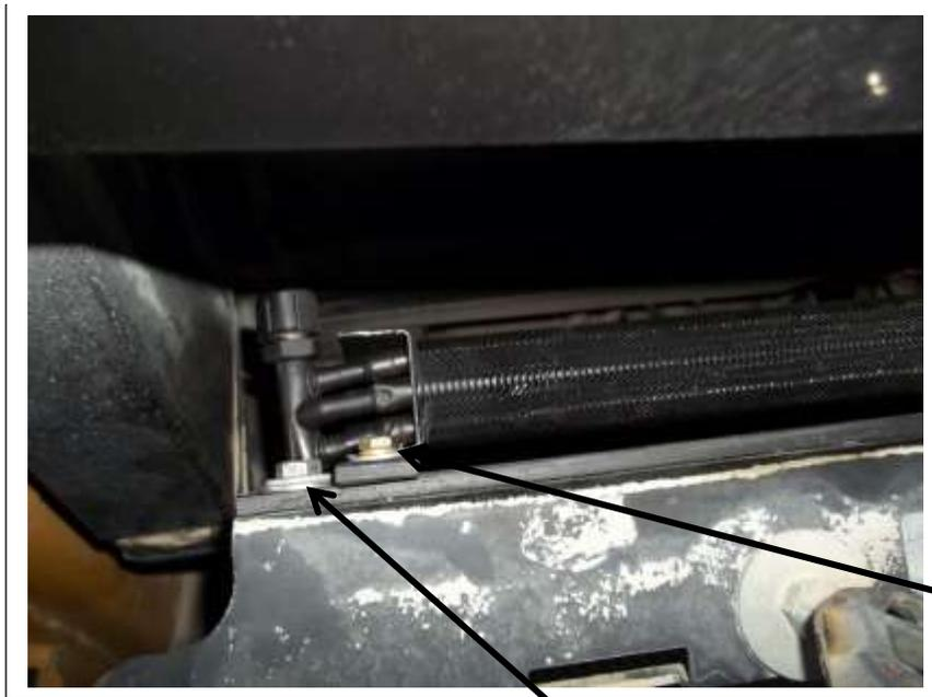
1/4" hardware bolting condenser to top bracket.
