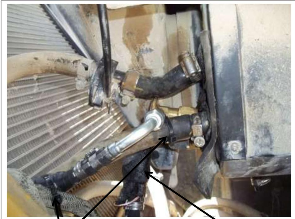
Secure all lines to prevent breakage from vibration
