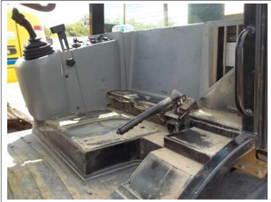
Remove the seat, left hand storage box and upper section of the floor liner. Remove the bolts from the lid of the heater blower box to access the interior.
