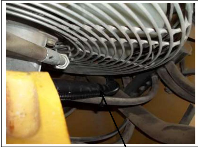
1/2" hose and clutch wire running beside the radiator fan and out of the engine compartment to the right of 3 or 4 hydraulic lines. The hose will come out just over top of the right rear axle.
