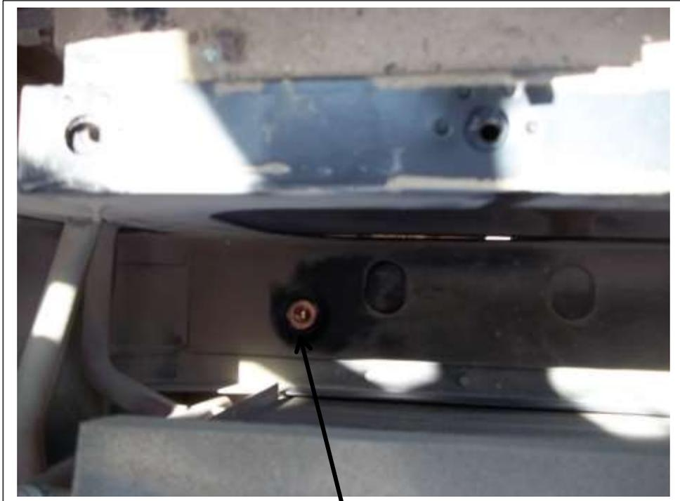
Drill out to 9/16" the two existing holes as shown and install the glue-in drain tubes into the bottom of the heater box. Use fast dry epoxy to glue in.
