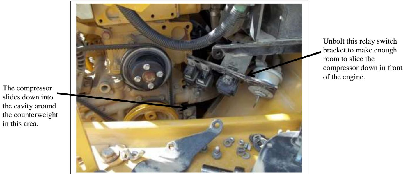
Remove the cover to get access to the area where the compressor will be located. Removing the taillight assembly is a must.
