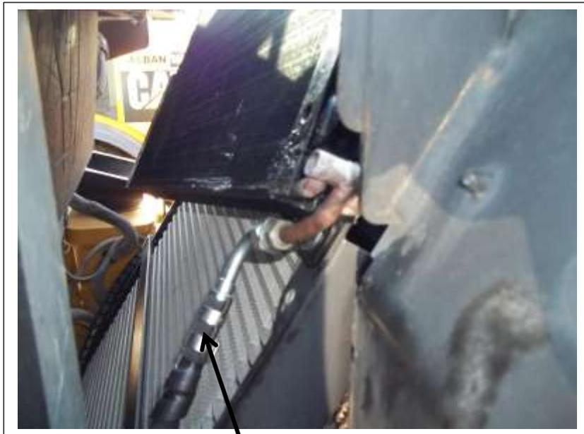
5/16" hose ( 64" long) mounted on the bottom fitting of the condenser going over to the drier on the right side of the radiator.
