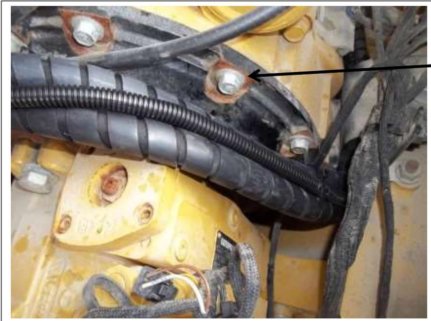
Use this bolt to secure the hoses with the double hose clamp supplied in the kit.
