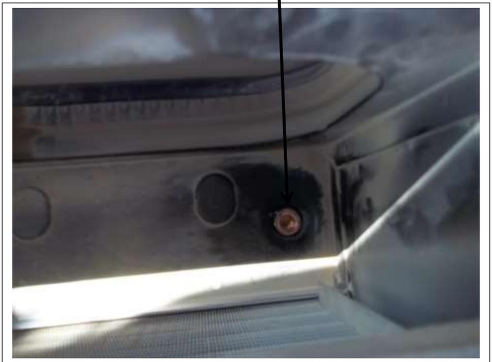
Install the short drain tube onto the copper extension previously glued into the box on the fitting end of the box. Add the drain tube restrictor and tighten the clamps.
