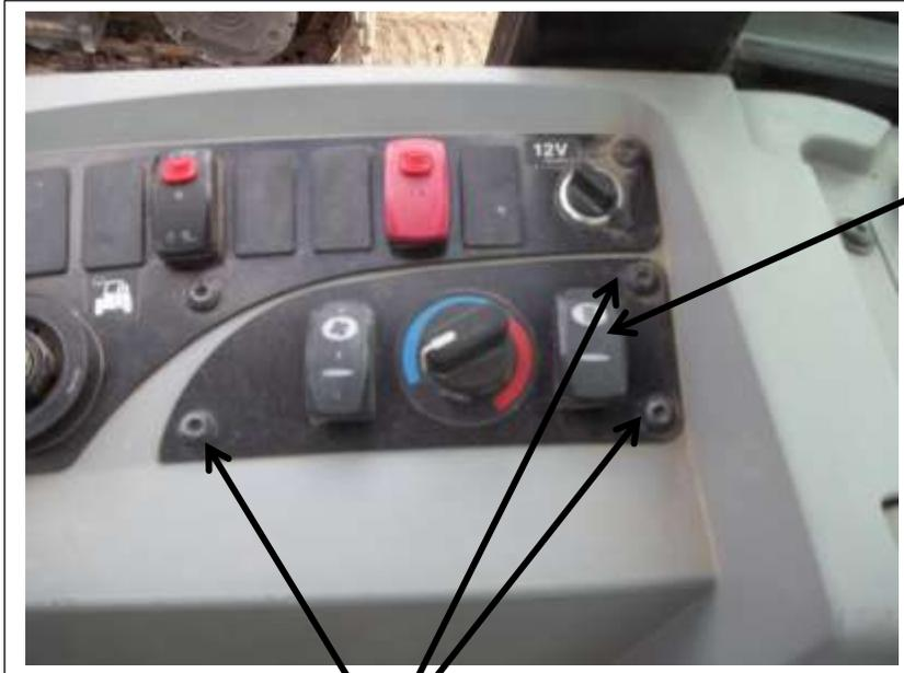
Replace this switch with new switch in kit
