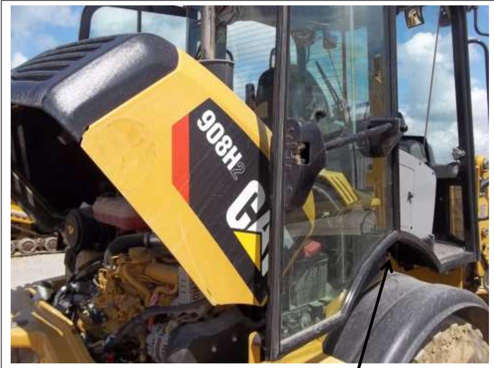
Remove this panel to get access to the heater hose connections. On the 906H2 machines, remove the plastic fender first.
