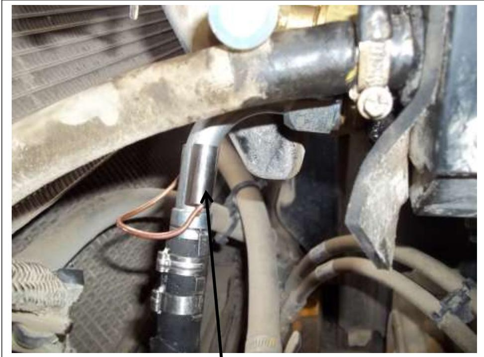
Expansion valve bulb clamp. Install as shown
