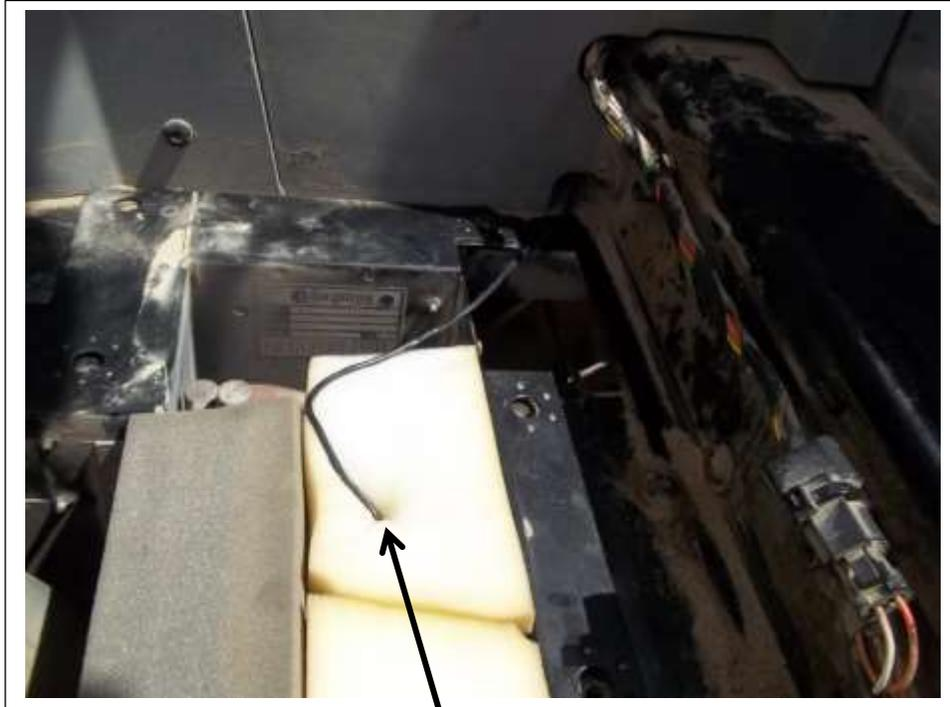
Insert about 6" of the thermostat probe into the evaporator coil as shown between the second and third rows of the coil. Note this area will already have the 1/8" foam on it. Install the probe through it as well.
