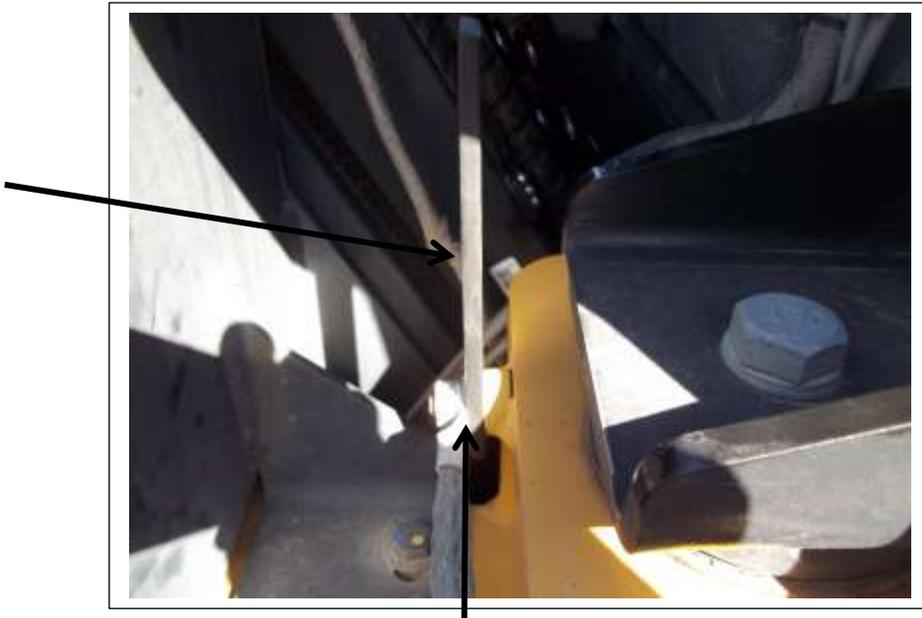
Bolt the drier bracket on the inside of the ground lug as shown.
