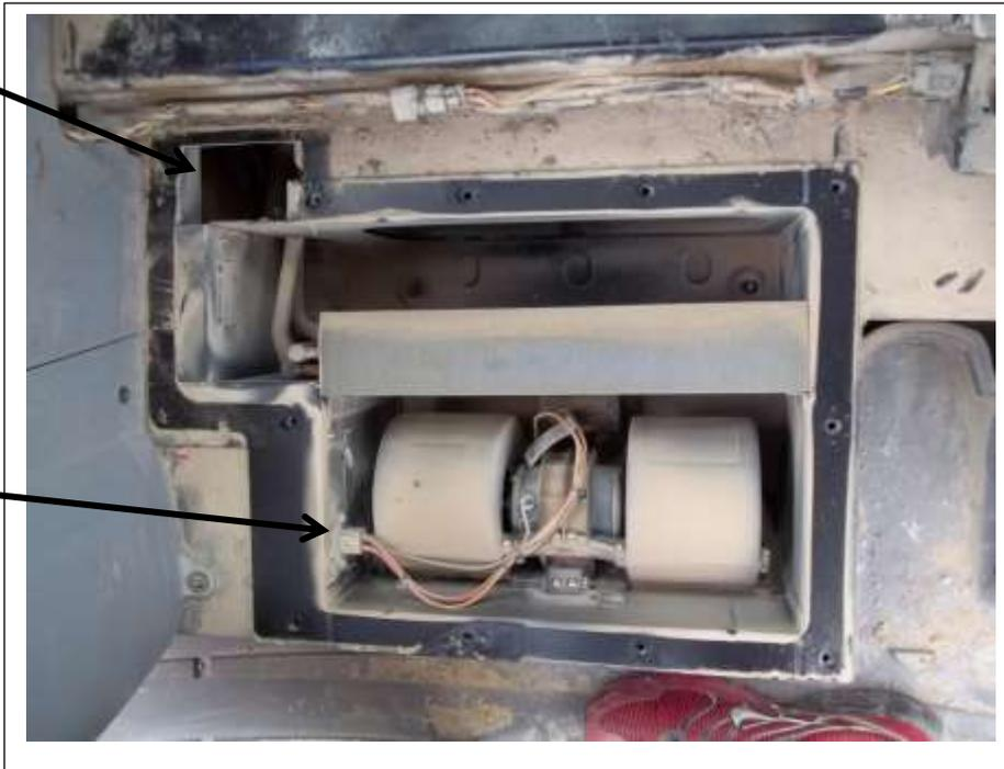
Lid removed. The blower box cannot be removed until the heater lines and blower wiring are disconnected. The access panel is on the side of the machine.
