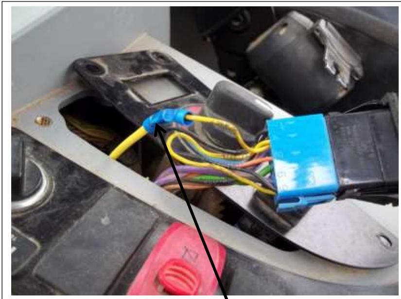
Butt connect the wire from the thermostat as shown, to the existing yellow wire # 521 that will be cut and stripped.
