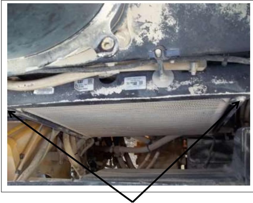
Remove these two bolts ( one on each side) at the top of the existing oil cooler.
