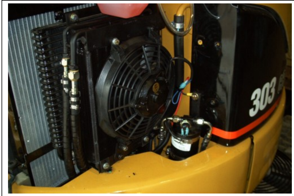
Condenser and drier with hoses.
