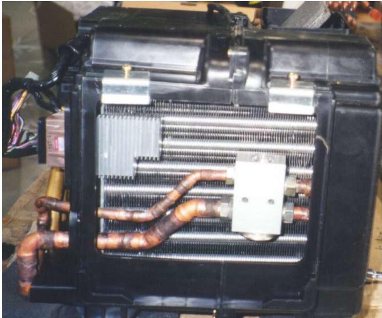
View of evaporator face showing expansion valve and supply lines out of box.
