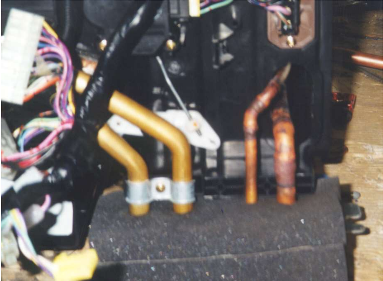
Side of evaporator housing assembly showing A/C tube routing out and down through seal material in floor.
