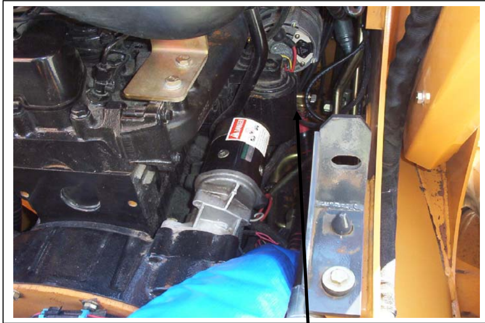
Water lines looping down under the engine and connected to heater tap.
