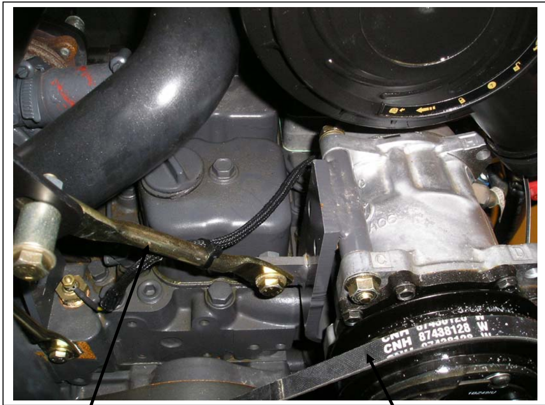
Compressor mount stiffener bracket.
