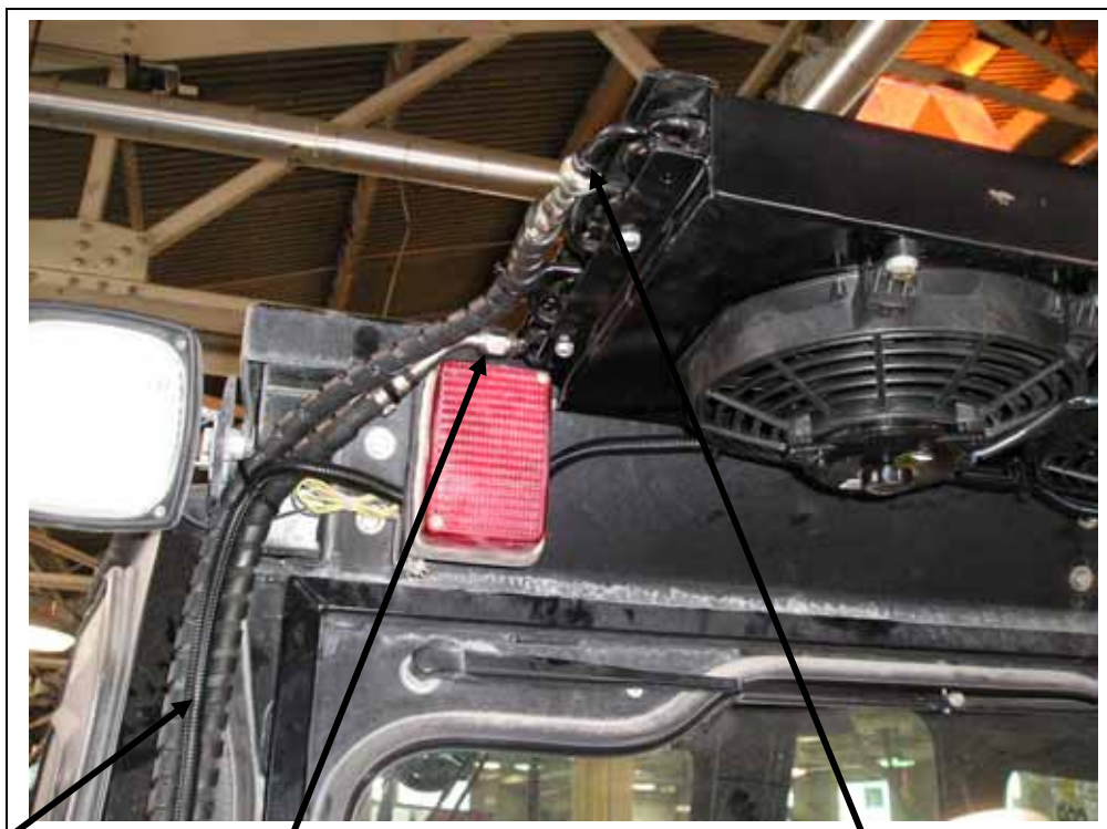
Right mount bracket. Bolt to cab roof.
