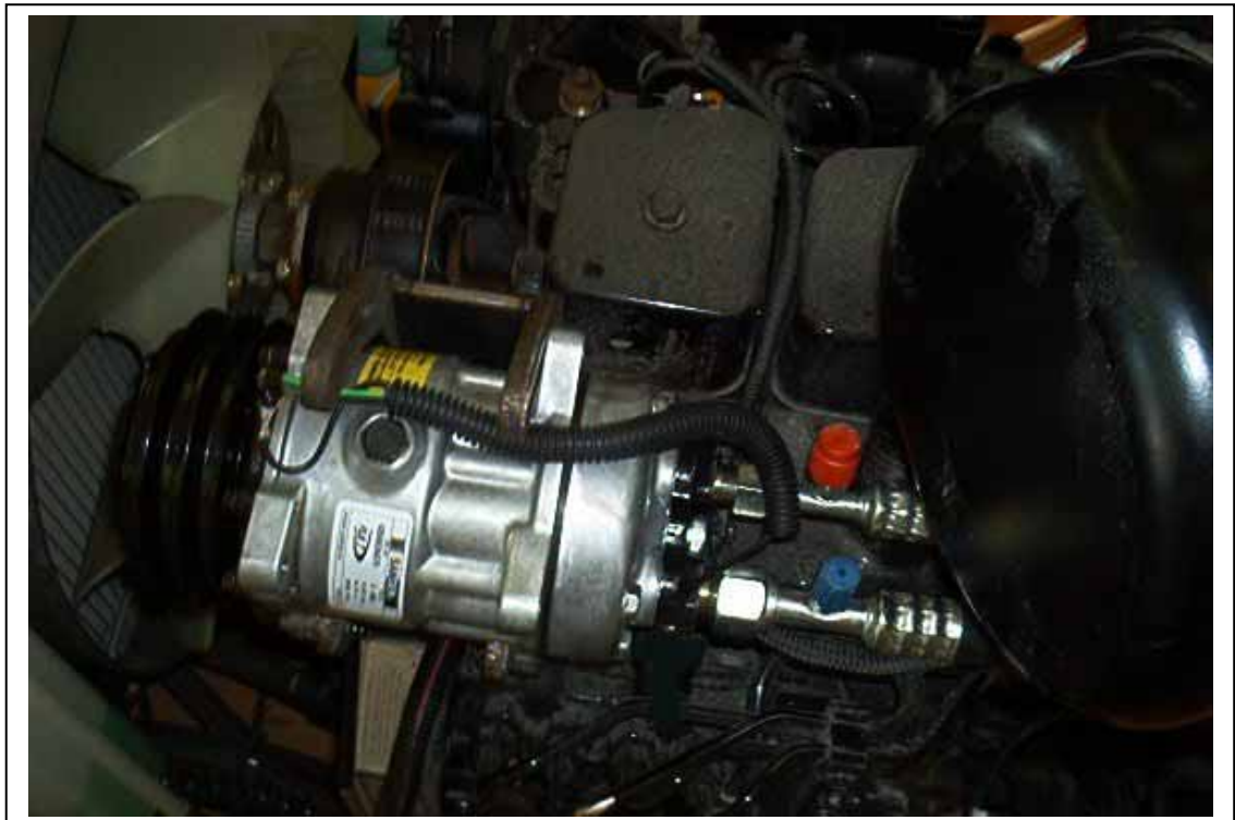
Binary switch mounted on high side of pad fitting
