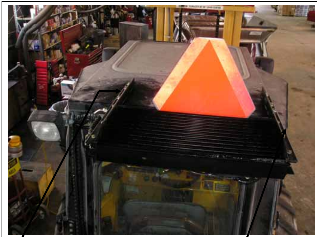
Left mount bracket. Bolt bracket to cab roof.
