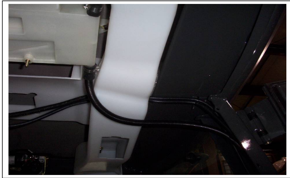
Left rear drain tube
