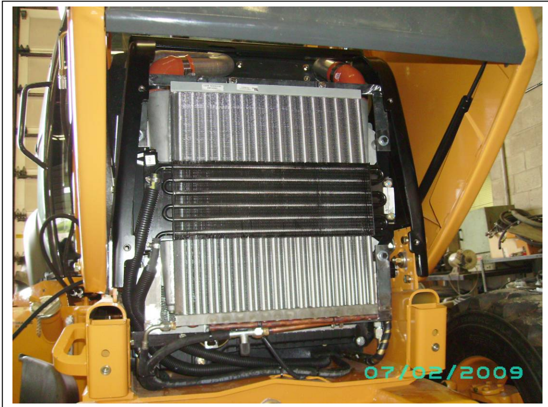
Condenser and hoses in place
