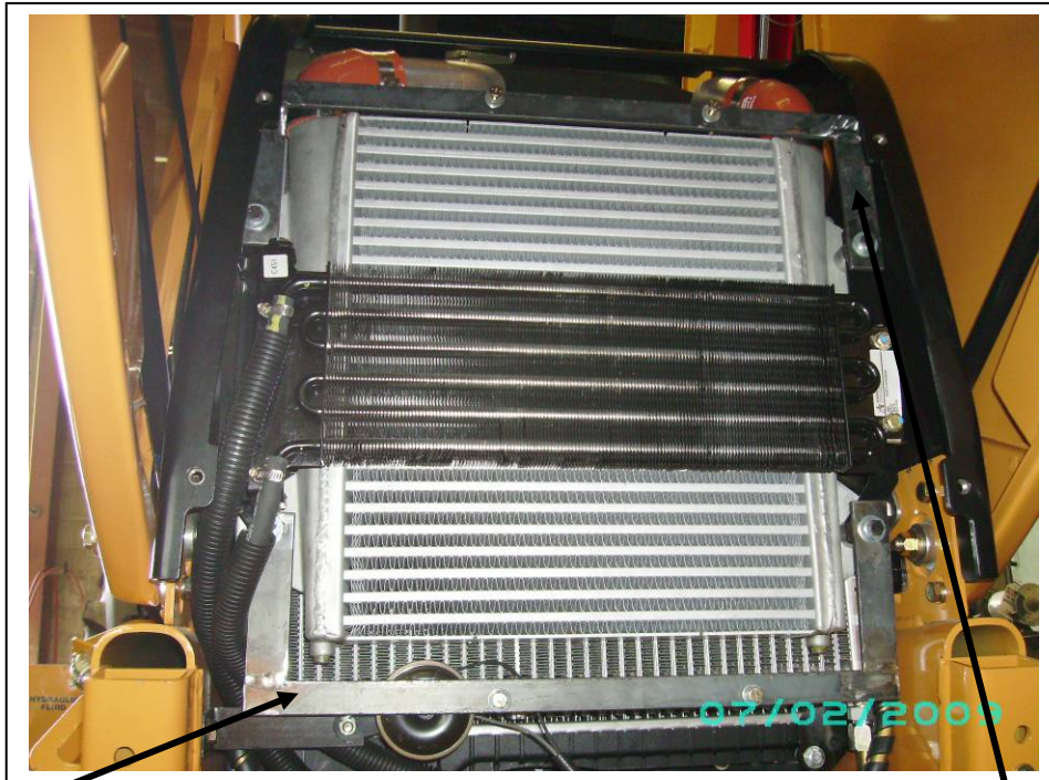
Lower condenser bracket in place
