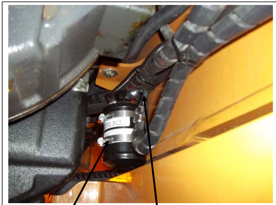
5/16" 90° fitting on the drier inlet.
