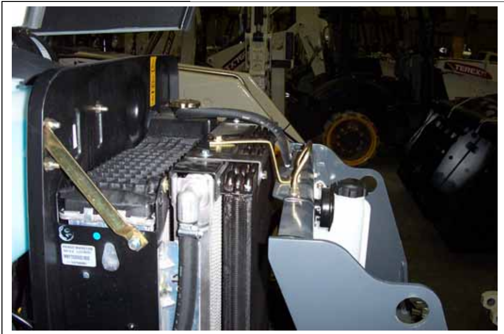
Side view of condenser installed
