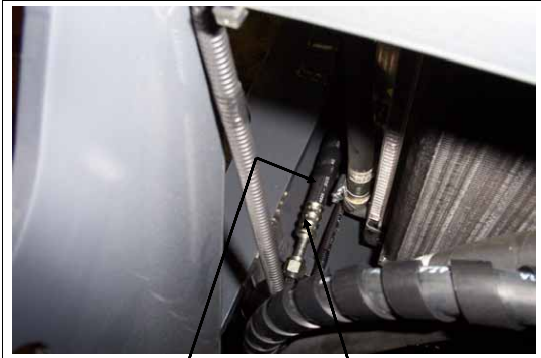
5/16" hose, drier to expansion valve
