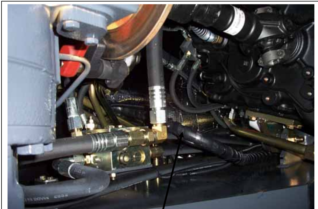
1/2" hose running up and over the rear axle and heading to the right side of the machine to the AC fittings at the heat/AC box.
