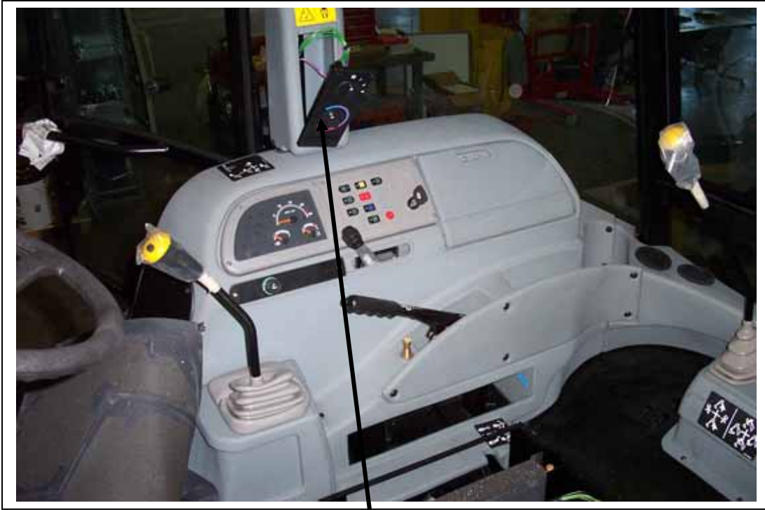
Heat/AC control panel unscrewed from frame
