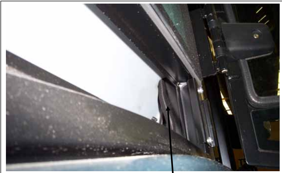
Clutch wiring running up into the control panel area. Wire loom will not fit up. Outside air filter removed to access this area.
