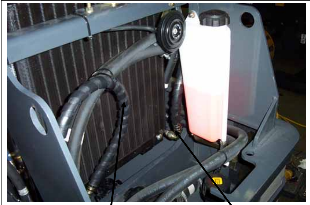
5/16" hose from condenser to drier
