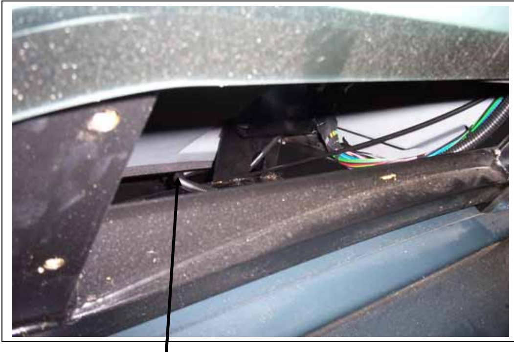
Clutch wire running down from the control panel towards the thermostat location. Looking down through outside air filter hole.
