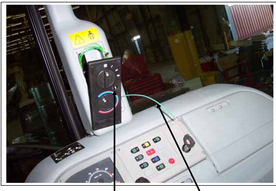
5/8" hole drilled for AC on/off pushbutton switch
