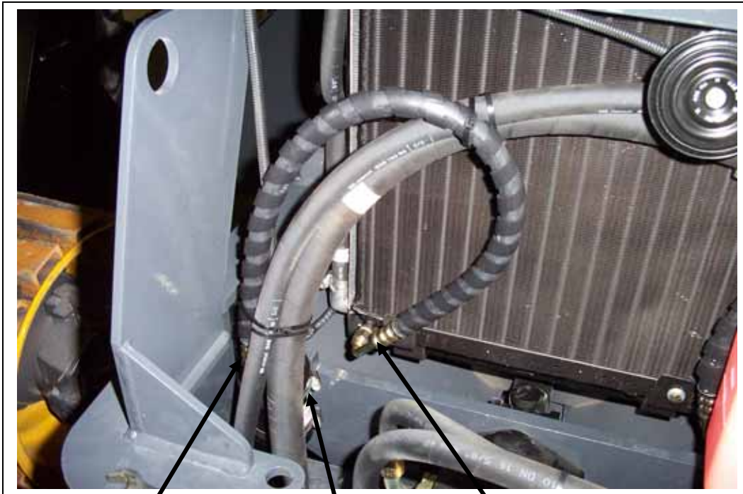
5/16" 90° fitting at drier inlet
