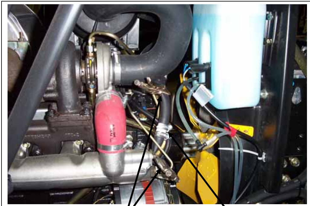
Clamp off heater lines on both sides of splice
