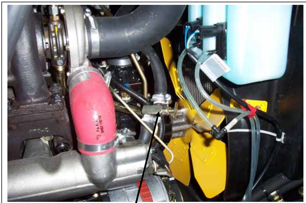
Heater line splice removed and replaced with heater line shut off tap.
