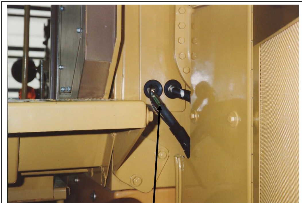
Hose and clutch wire entering the cab.
