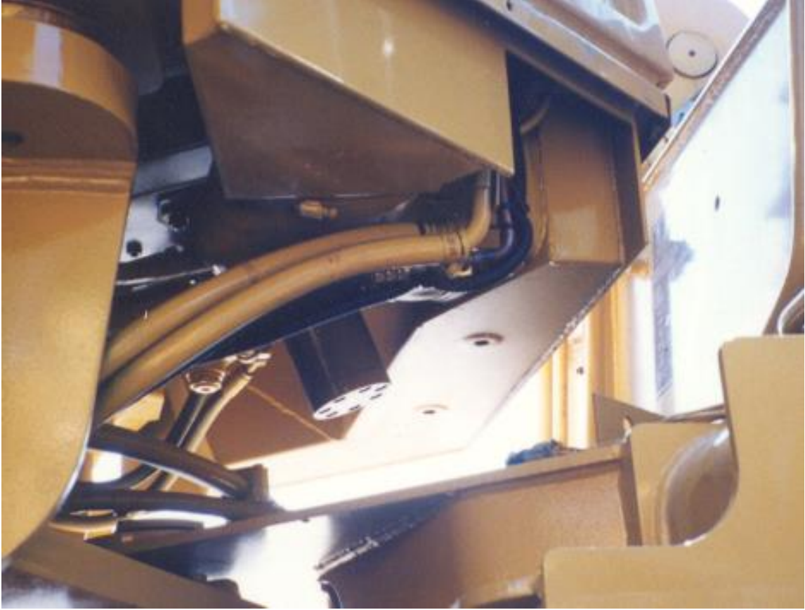
Hoses under cab.
